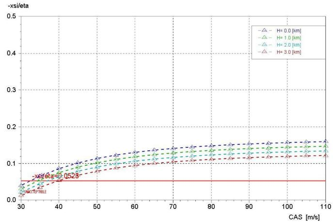
Dutch roll characteristics versus calibrated airspeed (CS-23.181 criterion) 4th EASN Association 20/37 International Workshop
