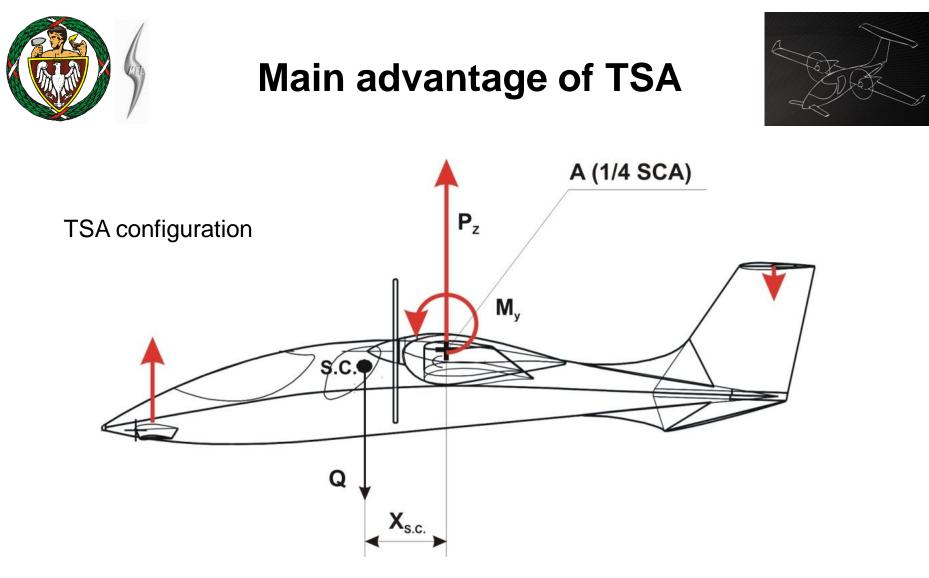
Additional 3<sup>rd</sup> surface decreases negative lift on the horizontal tail and improves the lift balance and classical horizontal tail satisfies longitudinal stability
