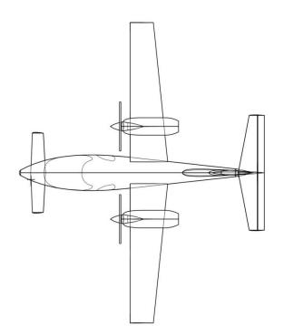
Wingspan 11.0 m Length 9.0 m Height 3.0 m Wing area 12.5 m2 Max. TO weight 1280 kg W/S 103 kg/m2 Engines power 230 HP Minimum airspeed 90 km/h Cruise airspeed (at sea level) 280 km/h Cruise airspeed (at 14000ft) 320 km/h Ceiling 18000 ft
