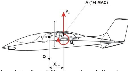
The neutral point of stability can be defined as the point which satisfies condition, that pitching moment coefficient is constant versus angle of attack or lift coefficient:
