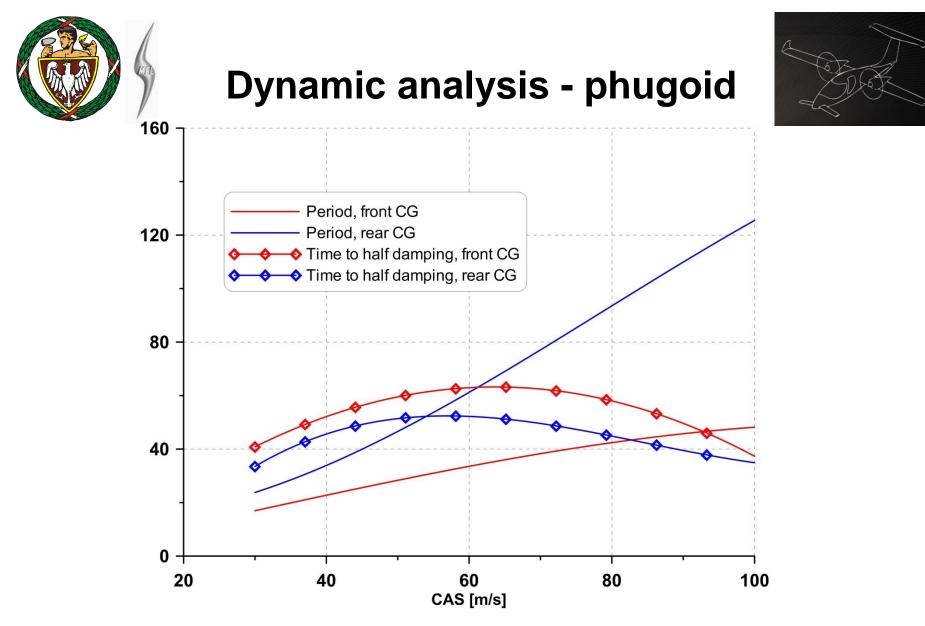
Phugoid - period and time to half damping versus calibrated airspeed
