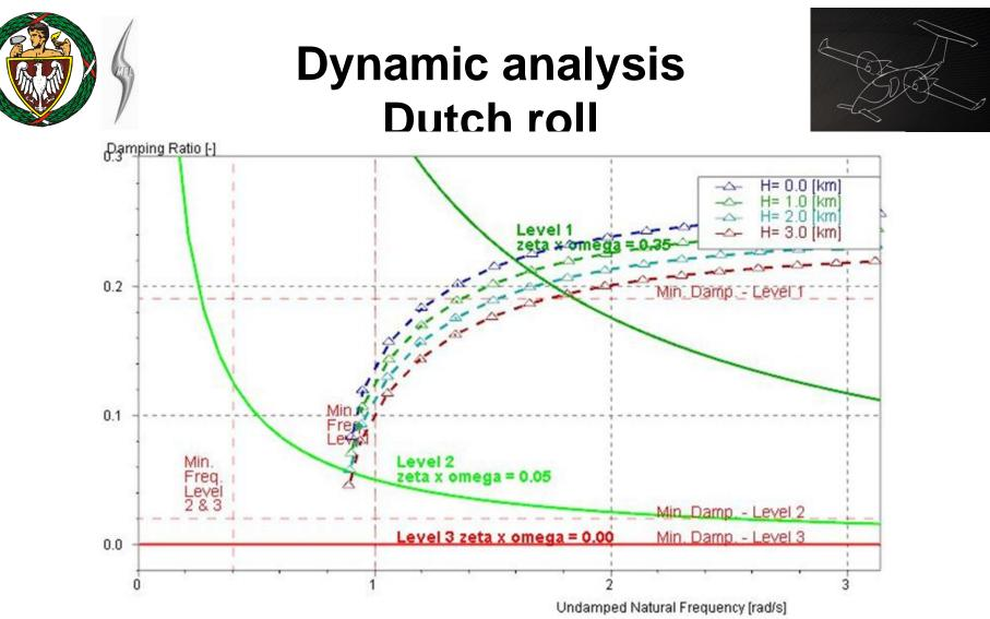
Dutch roll characteristics against background of MIL-F-8785C for landing configuration and rear CG position criteria. It also shows good Dutch roll characteristics, which are in Level 1 & 2 for whole flight envelope.
