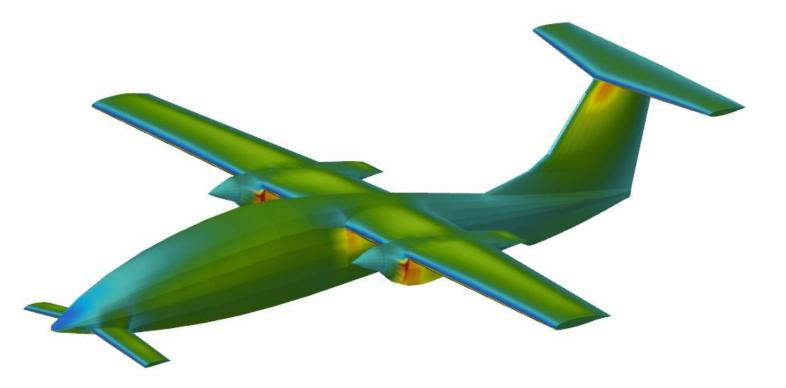
New configuration of AT-6 - example of pressure distribution (PANUKL), angle of attack  $\alpha$  = -5°
